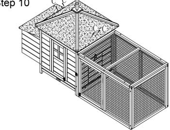
Put the whole roof to house, secure roof with 4x screw C according to pre-drilled holes as pictured.
