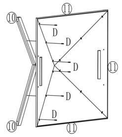
Connect 4x part (1) as shown, attach 4x part (10) outside part (1), and secure with total 24x screw D from inside. Better to finish one by one.
