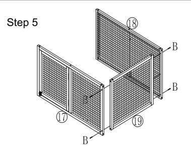
Connect part(17), part(18), and part(19), secure with 4x screw B as pictured.
