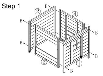
Connect part①, part②, part③ and ④, secure these four parts with 8x screw B as pictured.
