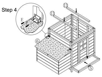
Attach part⑥, secure each hinge with 2x screw E; put in two perches part⑥andthen insert metal tray part⑤
